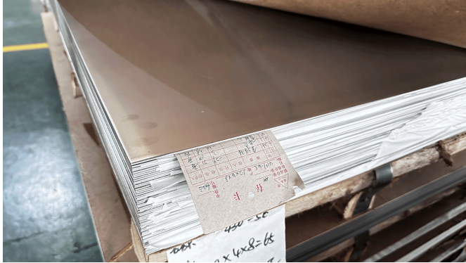
Cold-rolled stainless steel sheet metal
