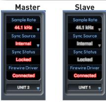
Sample rate and digital sync settings can only be set when Saffire MixControl has control of the Master Sync Device. When controlling the slave device, sample rate and sync status are greyed out.
