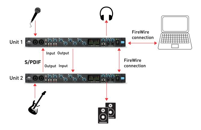
When you have connected your hardware as shown, you will then need to configure your software. If you want to monitor all of your inputs from the outputs of both units (as pictured above), both units will need 2 output mixes configured.
