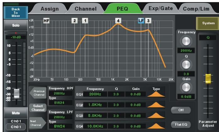
Figure 4.2: PEQ Parametric EQ Screen
