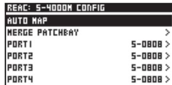
2. Select the port from "PORT1" to "PORT4" where the device you want to change is connected, then press [ENTER].
