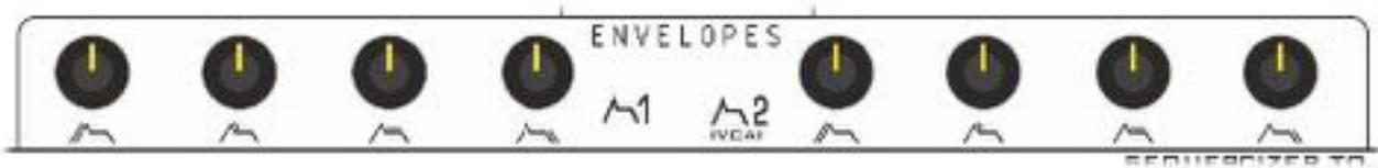
Impulse Command features two separate analogue ADSRs envelopes.
