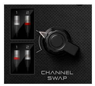
Channel swap – this function is exclusive to Edge Duo, since it uses two inputs. It allows you to switch the channel order F-B (L-R) or B-F (R-L).
