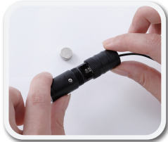
Unscrew the battery case
