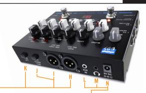
Note: The balanced outputs offers high-quality 'line box' signals for connecting to PA mixing consoles or to studio or broadcast recording units, with high noise immunity. The output level controlled by the MASTER knob does not affect these outputs.
