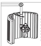
The microphone screen may be used with a studio boom that features a down extension. Assembly is the same except the screen and microphone are inverted.
