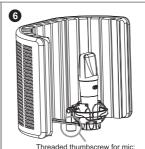
If your microphone is too long, you can directly connect microphone to threaded thumbscrew for microphone (D) without connect to the extension stand with thread (E).
