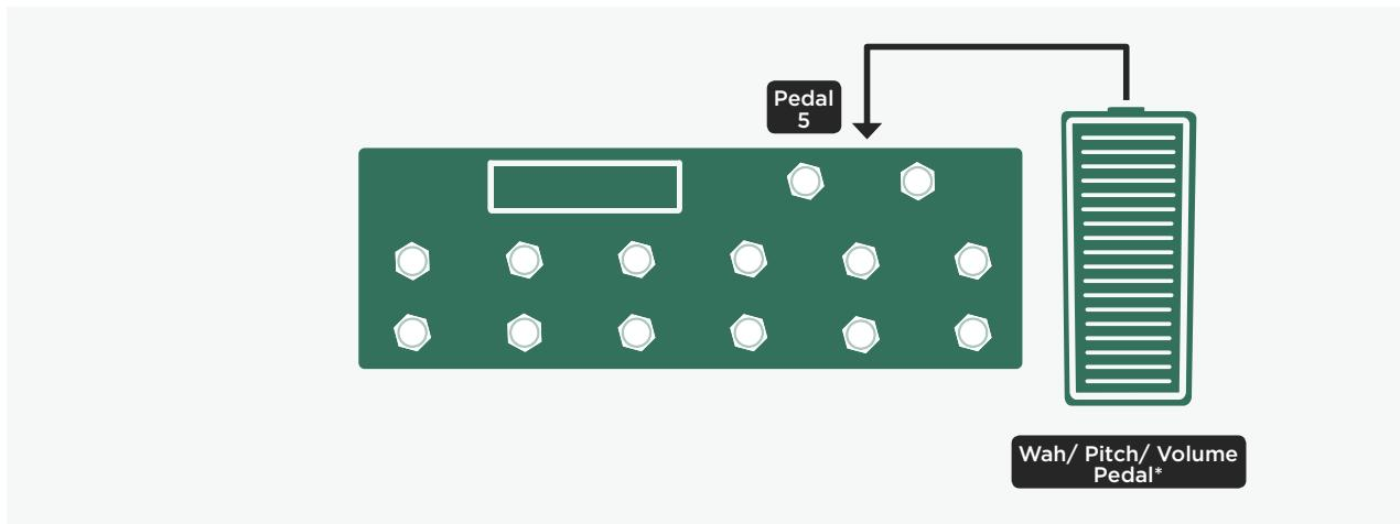
\* Wah Pedal also controlling Pitch and Volume („WahPedal to Pitch“ and „WahPedal to Volume“); Morphing triggered via buttons.
