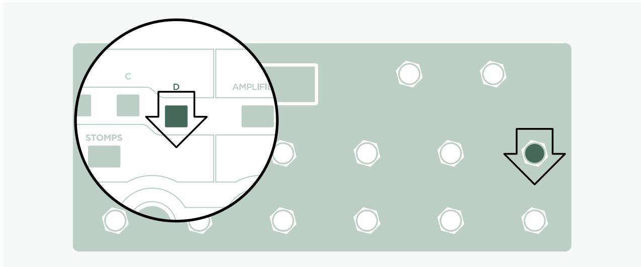
Assigning switching functions to the Effect Buttons is simple: just press and hold an Effect Button on the Remote for example Effect Button IIII and press the desired module button, e.g. Module D, on the front panel of the PROFILER at the same time. Done!
