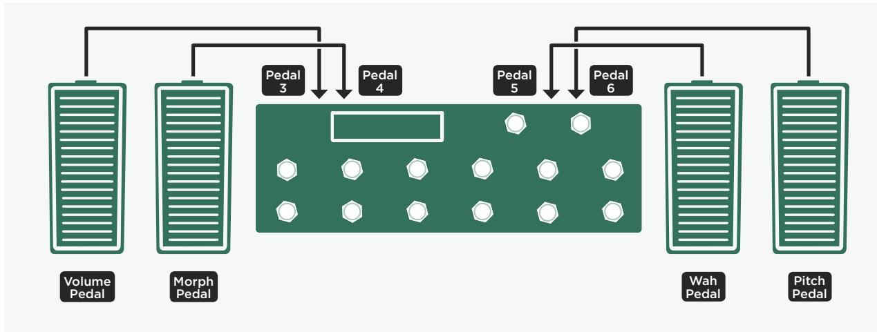
The Remote offers four TRS-sockets named “PEDAL 3” to “Pedal 6” to connect expression pedals. Their functions can be assigned in the System Settings of the PROFILER, as described in the “Expression Pedals and Foot Switches” chapter of the Main Manual and the “Expression Pedals” video tutorial.
