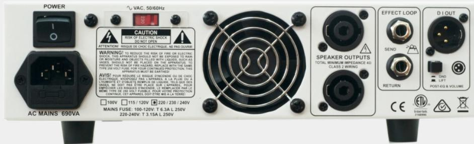
1. **On/Off Switch** Powers the Little Bass Thing on and off. Ensure this is set to the off position before connecting to mains.
