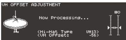
The "VH Offset" parameter is set automatically (approx. 3 seconds). The [TRIGGER] button stops flashing and remains lit.
