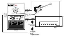
The Decimator II G String has 4 ¼ inch jacks. Connect the guitar directly to the Guitar IN. Connect the Guitar OUT to the input of the amplifier. Connect the DEC IN to the loop send and DEC OUT to the loop return. For best performance place all gain pedals in front of the amplifier and DEC IN. You can put Delay and Reverb effects pedals after the Decimator II G String and before the loop return to avoid cutting off reverb and delay tails.
