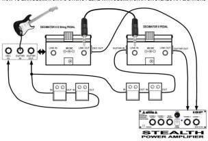
This diagram shows just one example of how to connect a Decimator II G String pedal with a standard Decimator II pedal for true Stereo A true stereo applications. Decimator system can realized by linking a Decimator II G String and a standard Decimator II. The above Diagram shows how to connect two pedal chains in Stereo. There are countless True Stereo this Applications: Diagram simply shows illustration of how to connect the two Decimator II pedals for true stereo use.
