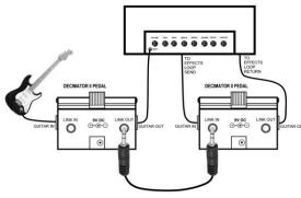
The diagram on the left shows how to LINK two Decimator II pedals allowing the second pedal to track the direct instrument input. This will allow the second pedals' internal level detector to track the guitar directly, providing tracking performance similar to the professional rack mount Decimator ProRack G. Connect an RTS 1/8 inch cable from the LINK OUT of the first pedal to the LINK IN of the second pedal.
