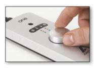
The controller knob operates in parallel with any software output controls.
