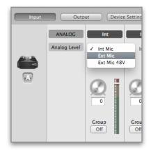
Select the Analog Level setting that corresponds to the microphone source you'd like to record. For example, if you have a microphone connected to the XLR connection on the breakout cable, select **Ext Mic** from the Analog Level menu on channel 1. If you would like to utilize ONE's built-in microphone, select **Int Mic**. Channel 2's source is always the 1/4" Instrument input.
