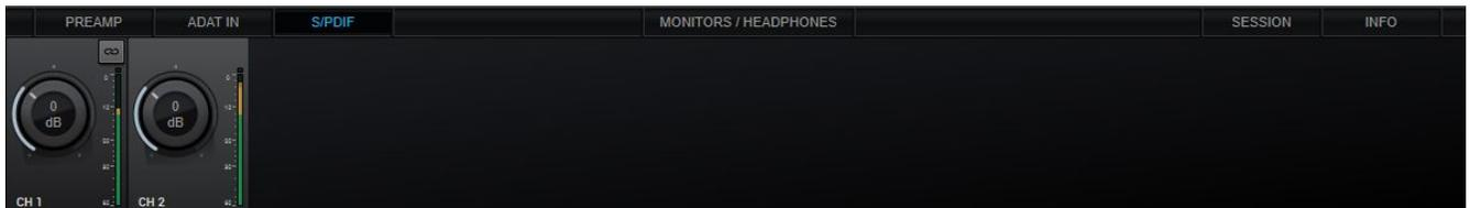
This tab contains controls for 2 S/PDIF digital audio inputs with editable text labels, gain adjustment knobs, Link buttons and signal meters. The available input gain range for all channels is -6dB – 12dB.
