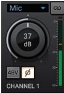
You will notice 12 large knobs labeled 'CHANNEL 1 – 12' in the 'PREAMPS' tab. Click the drop-down menu for CHANNEL 1 and choose 'Hi-Z'. Adjust gain by playing guitar while clicking and dragging the knob. Yes, it's possible with just one pair of hands. Yes, it's awkward.
