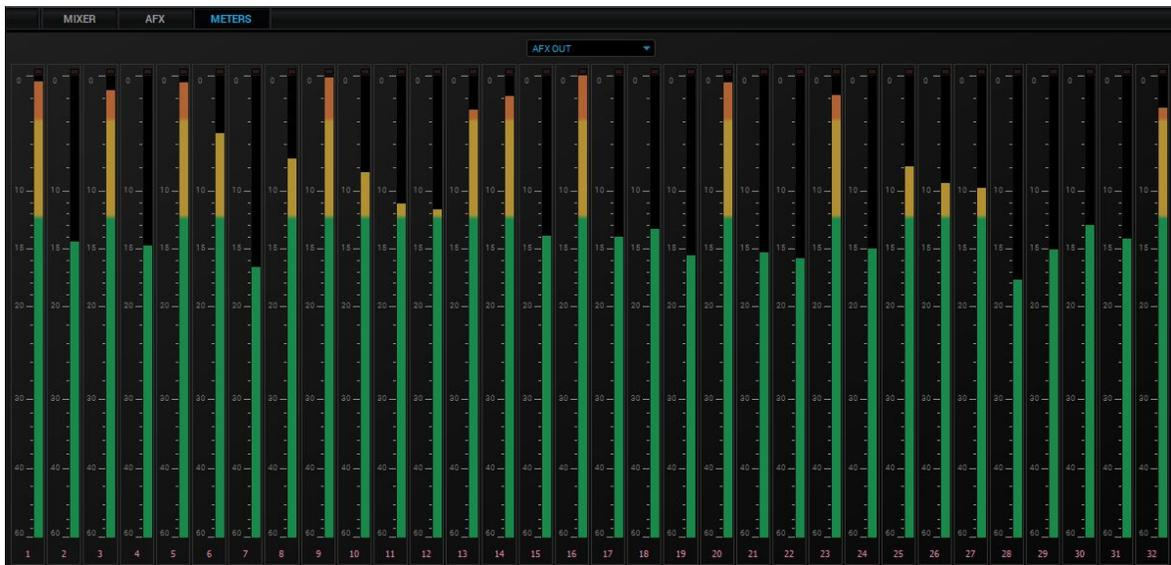
The Meters tab provides up to 32 individual volume meters for each row from the 'Routing' tab, selectable from the drop-down menu. Note that you can right-click (Command + Click on a Mac) to detach the Meters tab and have it in a separate window.
