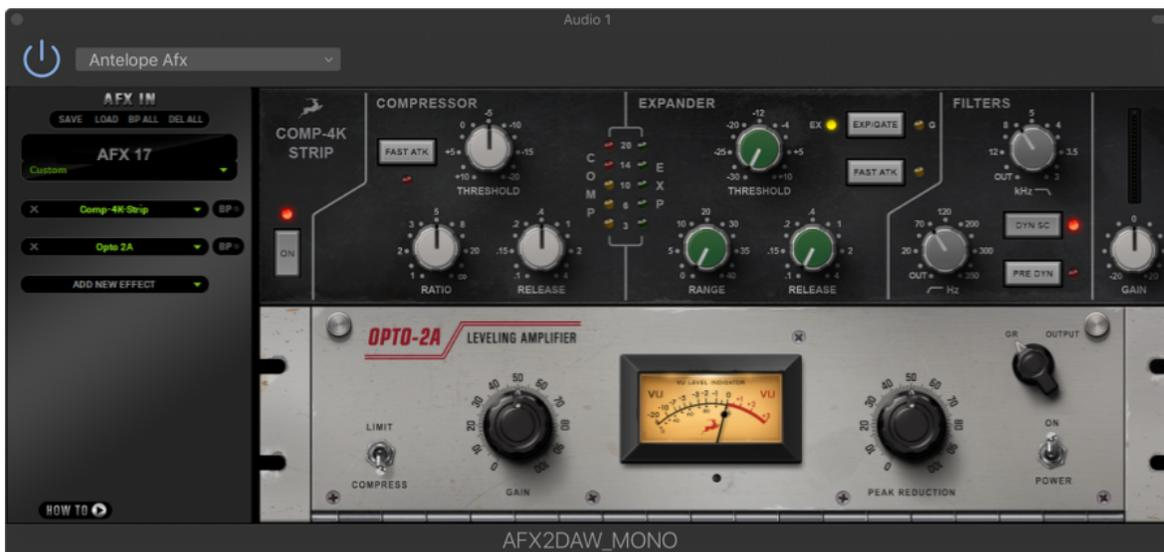
Available as a separate purchase, AFX2DAW is a bridge plug-in for using Synergy Core FX as inserts in your DAW. All Synergy Core FX processing and I/O audio streaming activity is handled by the DSP and FPGA processors in your interface. AFX2DAW provides a more immediate workflow with the added bonus of Synergy Core FX automation in your DAW, which isn't available otherwise.
