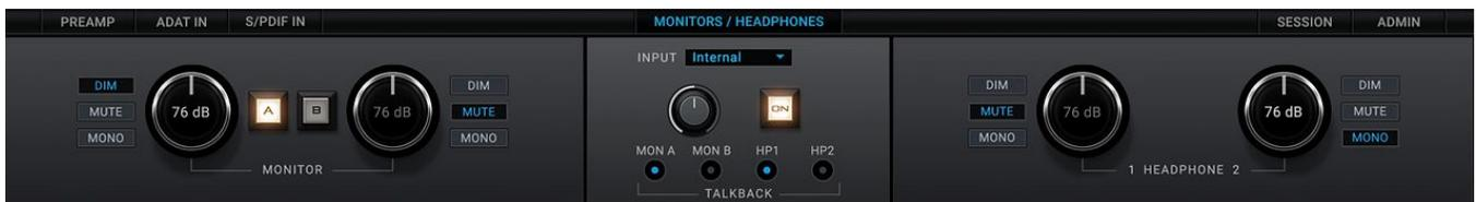
This tab has a dedicated monitoring control section for the monitor outputs, and controls for the headphone outputs, and the integrated Talkback microphone.
