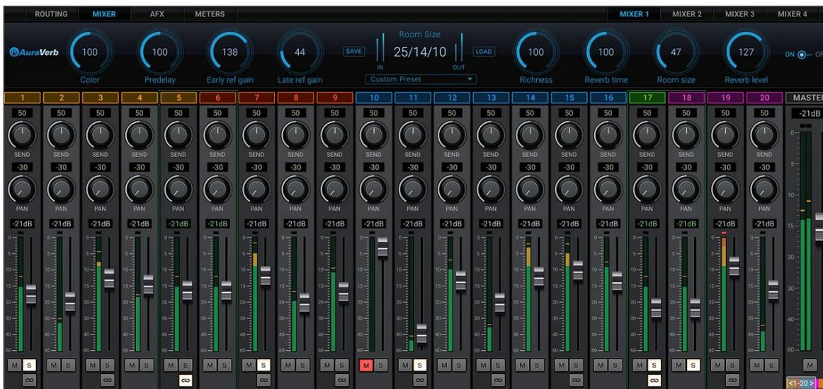
The Mixer tab is home to four 32-channel software mixers. Each channel is equipped with Pan, Volume, Solo, and Link controls (on odd-numbered channels), as well as metering. The Master channel has Volume and Mute controls.
