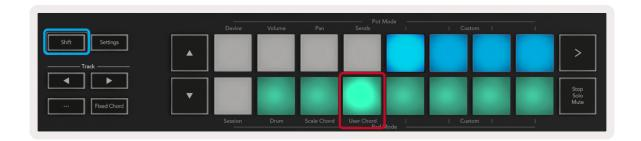
To assign a chord to a pad simply press and hold the pad and press the notes that you want to assign from the keyboard. Up to 6 notes can be assigned to each pad and can be input with individual pushes of the keys, meaning you do not need to hold down all the notes at once so long as the pad is being held.
