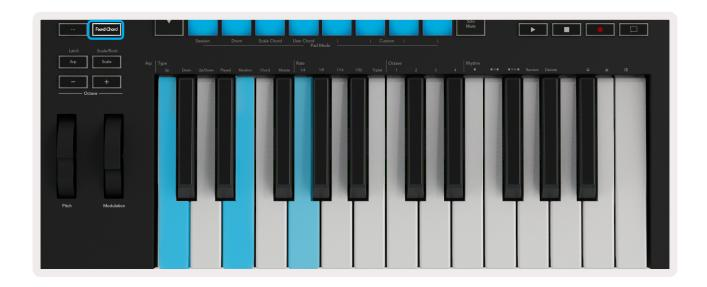
Press and hold the Fixed Chord button, then press and release C, then E, and finally G (a C Major chord). The unit stores this as the 'fixed chord'. Release the Fixed Chord button.
