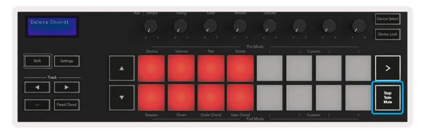
You can lock the chords using the scene launch button. Locking the chords allows you to play keys and the pads without risk of overwriting your chord assignments. Pressing the scene launch button toggles between locked (lit blue) and unlocked modes (lit white).
