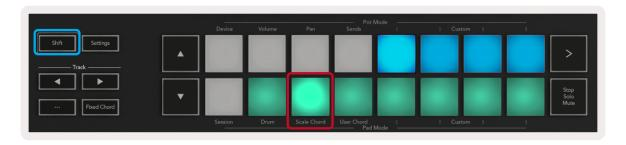
The first and last pad of each row light up more brightly than the middle pads to indicate root chord position. To navigate between pages of chords use the ▲ ▼ navigation buttons. On the first page the top row of pads are lit blue and contain triads, the bottom row of pads contains 7ths and is lit a darker blue. Pressing the ▼ button will reveal a row of 9ths, with the pads lit up in purple, below this are 6/9ths and the pads will light up in pink.
