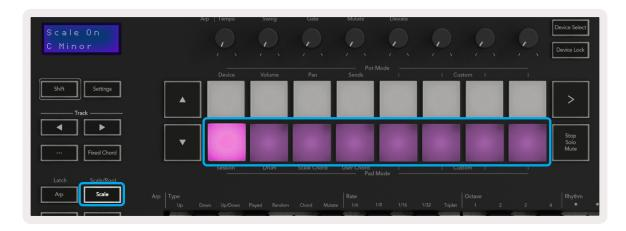
The bottom row of pads will be lit and can be used to select a scale, the selected scale is then shown on the screen. From left to right the pads can be used to select the following scales: Minor, Major, Dorian, Mixolydian, Phrygian, Harmonic Minor, Minor Pentatonic and Major Pentatonic.
