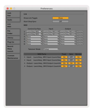
In the Link/MIDI tab you'll need to copy the settings shown above. First, select your Launchkey MK3 from the Control Surface menu. Then, under Input select "Launchkey MK3 [...] (LKMK3 DAW OUT)" or Launchkey MK3 MIDI IN2 (Windows) for output select "Launchkey MK3 [...] (LKMK3 DAW IN)". Finally, match the Track, Sync and Remote settings.
