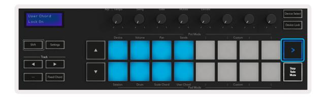
The ▲ ▼ buttons can be used to transpose the chord bank in semitones between -12 and +12, any changes will be displayed on the screen.
