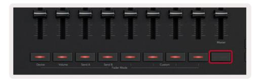
When set to Select the colour of the buttons will match the tracks in Live. Pushing a Fader Button (highlighted blue) will select that track.
