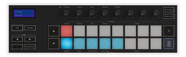
The two modes above are toggled by pressing the Stop/Solo/Mute button. Please note that when using Launchkey with Logic Pro the Stop/Solo/Mute button will only toggle between Solo and Mute modes, there is no Stop mode. Stopping the track is done with the Stop transport button.
