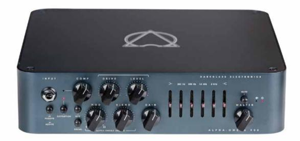
INPUT: Use this jack to connect your instrument via a standard  $\ensuremath{\mathcal{V}}_{\!\!4}"$  mono cable.
