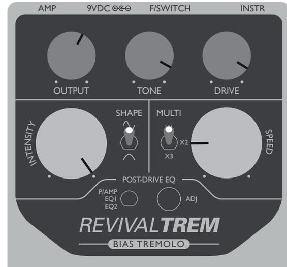
**Cranked Deluxe:** All out vintage overdrive! Pushing up the DRIVE control introduces a harmonically rich driven tone that's almost fuzz-like! Combine that with a high intensity, slow speed tremolo for some subtle modulation that creeps in as notes decay.
