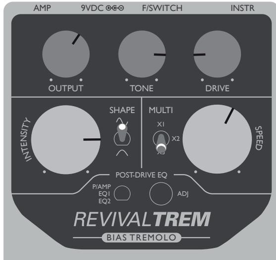
**Clean Tremolo:** The RevivalTREM cleans up nicely, just like an amp! In order to achieve a clean tremolo setting, dial back the GAIN control and compensate for any loss of volume with the OUTPUT control. These specific tremolo settings will deliver a faster, more intense effect.
