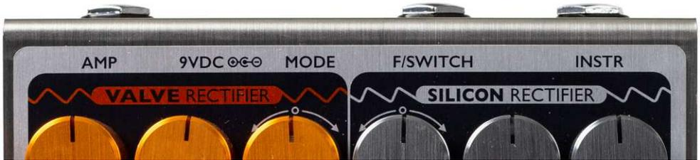
*Rear connections. Left to right: Instrument input; External Footswitch; Power; Output*
