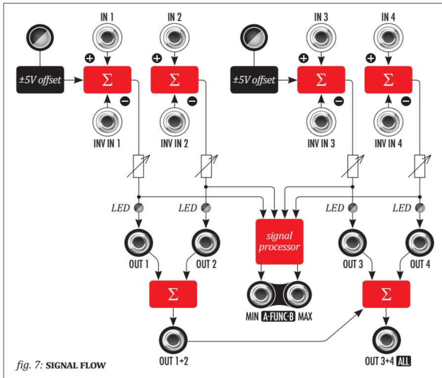
fig. 7: SIGNAL FLOW
