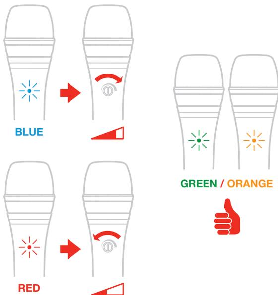
Please note the iRig Mic HD-A gain control is intentionally slightly recessed to minimize the risk of accidental level changes during usage.
