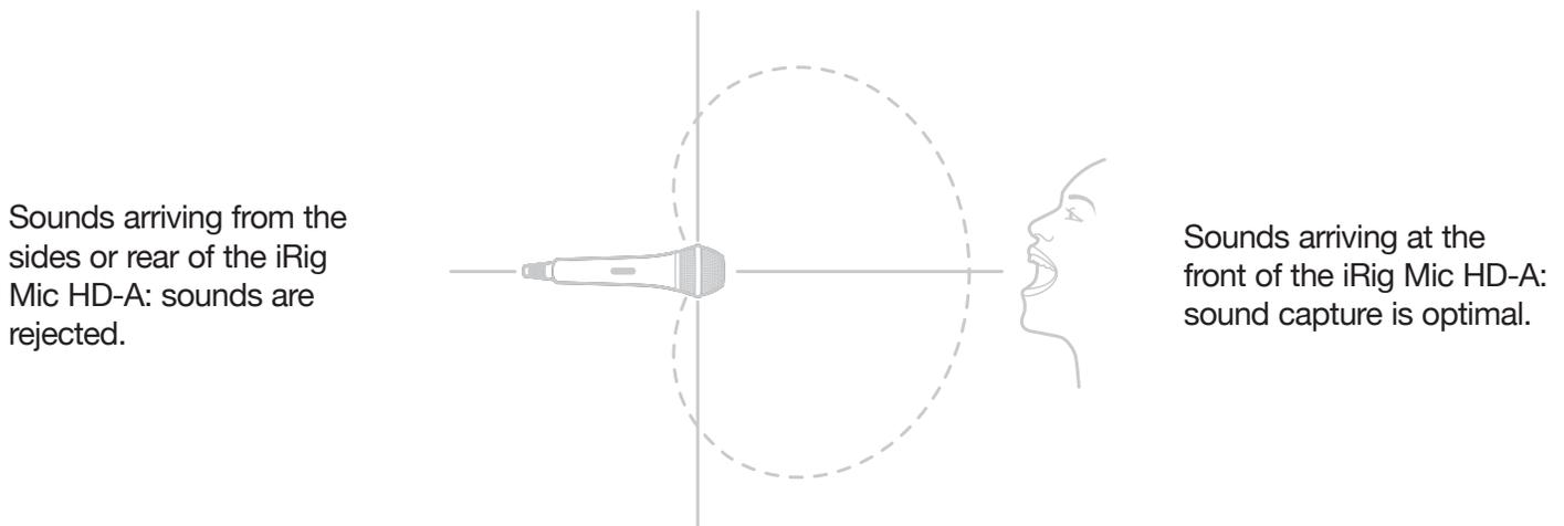
TIP: The built-in microphone of your mobile device is great for general recordings thanks to its "omnidirectional" pickup pattern. This means that sounds coming from all directions are captured almost equally. For this reason the iRig Mic HD-A is a great choice when increased clarity and isolation from unwanted sound is required.
