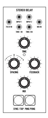
The Stereo Delay is, in fact, two individual BBD-based analog delays that share certain parameters. In the Matriarch signal path, the Stereo Delay is positioned after VCA 1 and VCA 2, and before the **MAIN AUDIO** outputs.
