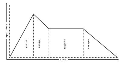
Regardless of how the Envelope is applied, there are four main stages: Attack time, Decay time, Sustain level, and Release time. These controls are identical for both Envelope Generators.
