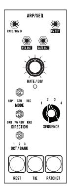
The Arpeggiator and multi-bank Sequencer are powerful tools for creation and live performance. In addition to the controls found in this module, the Arpeggiator and Sequencer also rely on the **PLAY, HOLD,** and **TAP** buttons located on the Left-Hand Controller panel. This module also contains the **CV OUT, VELOCITY OUT, GATE OUT,** and **ARP RATE / DIV IN** patch points.
