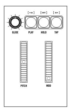
The Left-Hand Controller (LHC) is home to a number of performance-enriching controls. The **PITCH** (Pitch Bend) and **MOD** (Modulation) wheels deliver real-time expression, while the **GLIDE** knob provides enhanced articulation between notes. The Left-Hand Controller is also home to the Transport Buttons for the Arpeggiator and Sequencer, allowing instant access to these powerful features during performance.
