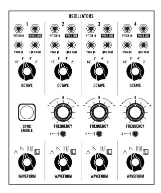
Matriarch's analog sound begins with four voltage-controlled oscillators (VCOs) of nearly identical design. Each oscillator provides individual control of the Octave and Waveform settings, while Oscillators 2, 3, and 4 also feature a **FREQUENCY** knob used for detuning from Oscillator 1.
