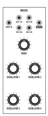
The Mixer is where all of the sound sources within Matriarch are blended together before being passed on to the Filter. Patch points in the Mixer allow each hardwired source (Oscillators 1 – 4 and Noise) to be replaced with an external audio signal. There is also a line-level Instrument Input on Matriarch's rear panel that feeds directly to the Mixer.
