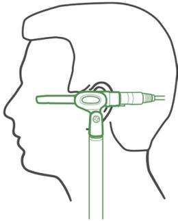
Example of correct ARC Condenser mic positioning:
