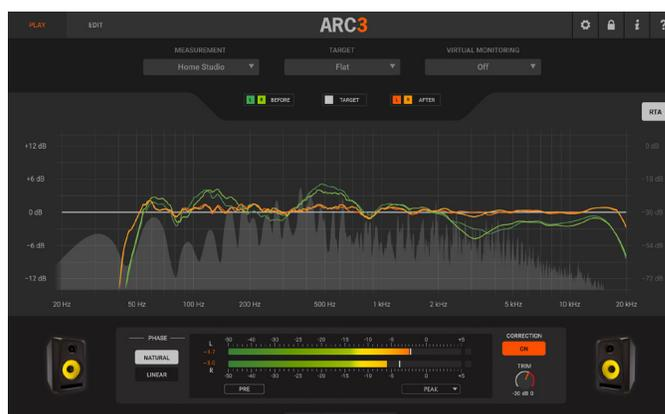
ARC System's MEMS microphone is calibrated and optimized to work with the software with a plus/minus 0.5 dB tolerance, allowing the system to work at its highest precision. However, ARC 3 will also accept profiles for other popular room analysis microphones if you already own one.
