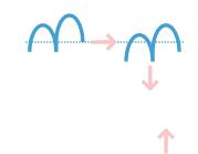
Overtone Output Jack Audio output of Modified Center Clipped waveform. This output explores removing the fundamental harmonic frequency by folding the top and/or bottom of the waveform in on itself. Also a nice way to turn a sine wave into the batman symbol. Overtone output is out of phase with Clipped Output Jack.
