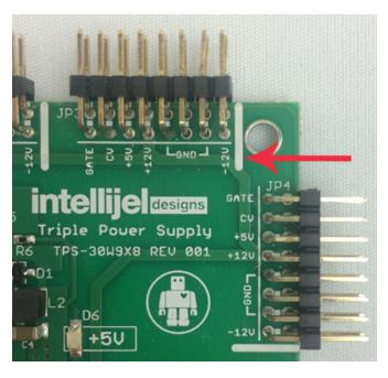
Most modules will come with the cable already connected but it is good to double check the orientation. Be aware that some modules may have headers that serve other purposes so ensure the power cable is connected to the right one.
