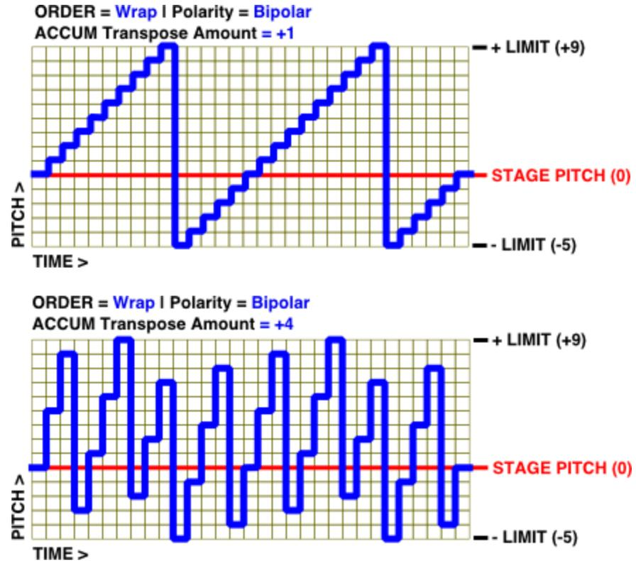
Pendulum Pitch accumulates in the direction set by the stage's TRANSPOSE AMOUNT. When the accumulated pitch reaches its Positive Limit (or Negative Limit), it reverses direction and continues accumulating in the opposite direction until it reaches either:
