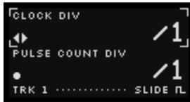
This button opens the DIV screen, which (for the selected track), divides the sequencer's global clock (internal or external), plus any stage-based Pulse gates.
