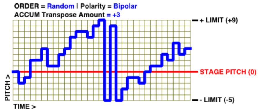
*NOTE: Since the 'drunken walk' can extend both above and below the stage pitch, and accumulations wrap to the opposite limit (rather than back to the stage pitch), this can result in some wider pitch swings — particularly when the 'walk' occurs near a limit.*
