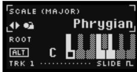
The built-in scales are a superset of those available in other Intellijel products, such as *Scales* and *Tête*, while also offering scales based on chord shapes, plus 100 user-definable scales.
