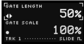
This button opens the TRACK GATE screen, which sets the selected track's default gate length for all the pulses (and ratchets) in the current track.
