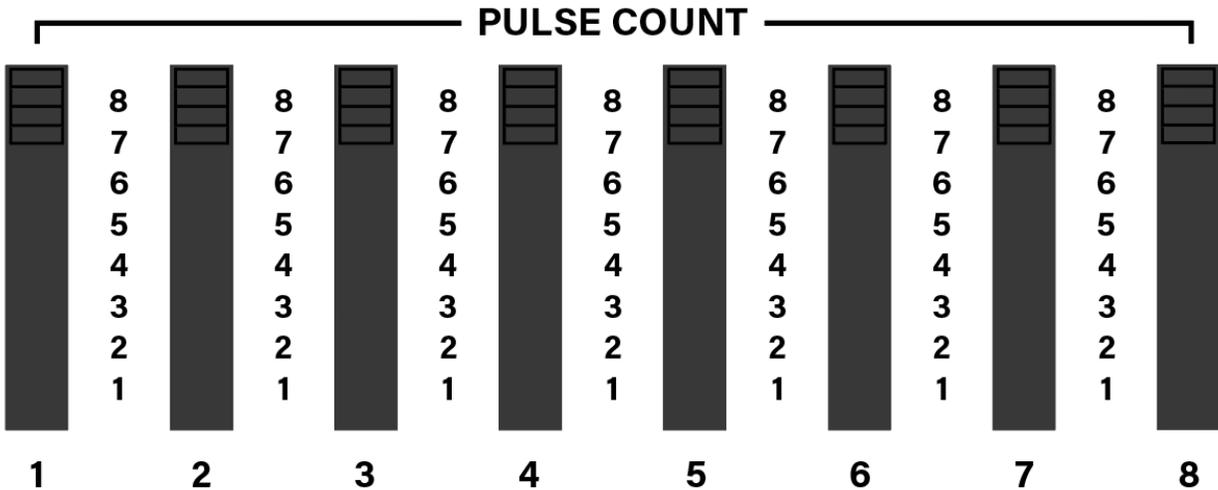
These switches set the number of clock pulses at which the sequencer stays on a particular stage. In general, the sequence will not advance to the next stage until the chosen number of clock pulses has passed. Each stage's pulse count can be set from 1 pulse to 8 pulses.
