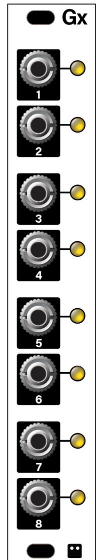
**Transport C :** **Gx/Qx** jacks 1-8 will output the following signals, and the `MX ASSIGN` parameter is not used.
