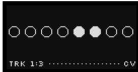
Each Stage has one of two gate states: on or off. Repeatedly pressing a Stage button toggles between setting that Stage's Gate value either high (5V) or low (0V). A high gate value (+5V) is indicated by a solid dot (along with a lit Stage button, when viewing the CV Lane). A low gate value (0V) is indicated by a hollow dot (along with an unlit Stage button, when viewing the CV Lane).
