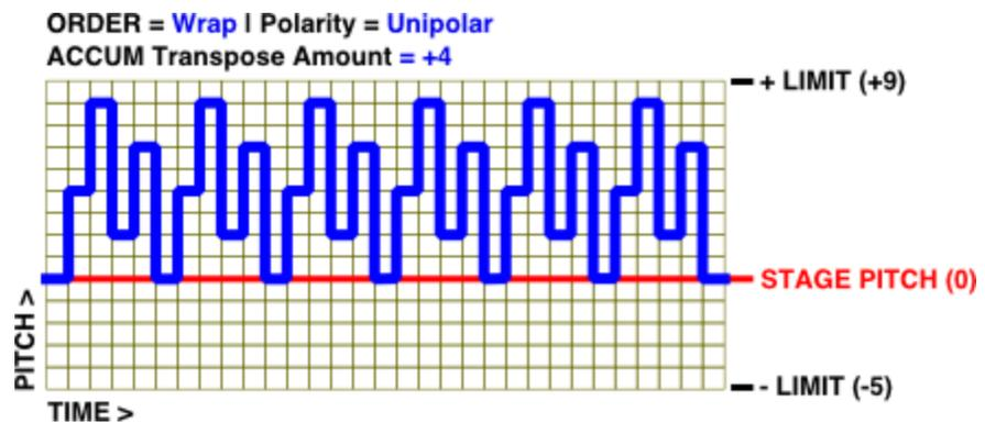
If you set a *negative* TRANSPOSE AMOUNT, accumulations will accrue in a downward direction beginning at the stage pitch; fall to the Negative Limit, then wrap back to the stage pitch and continue accumulating. No pitches above the stage pitch will occur.
