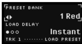
Banks are named by color. Selecting a bank causes all 8 Stage buttons to light with the chosen color. Each of the 8 Stage buttons corresponds to a Preset location in that bank. Brightly lit Stage buttons contain presets. Dimly lit Stage buttons are empty. A flashing Stage button indicates the most recently loaded preset (if you don't switch banks).
