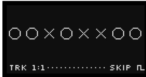
When SKIP is enabled for a stage, the sequencer treats the stage as if it did not exist — jumping past it to the next stage in the sequence (as defined by the [ORDER](#) screen). The stage's PULSE COUNT is also ignored completely, and does not count toward the total number of pulses in the sequence length.
