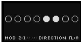
In the above example, we have assigned MOD Lane 2 to control the Playback Direction, which is a simple gate function, rather than a continuous voltage.
