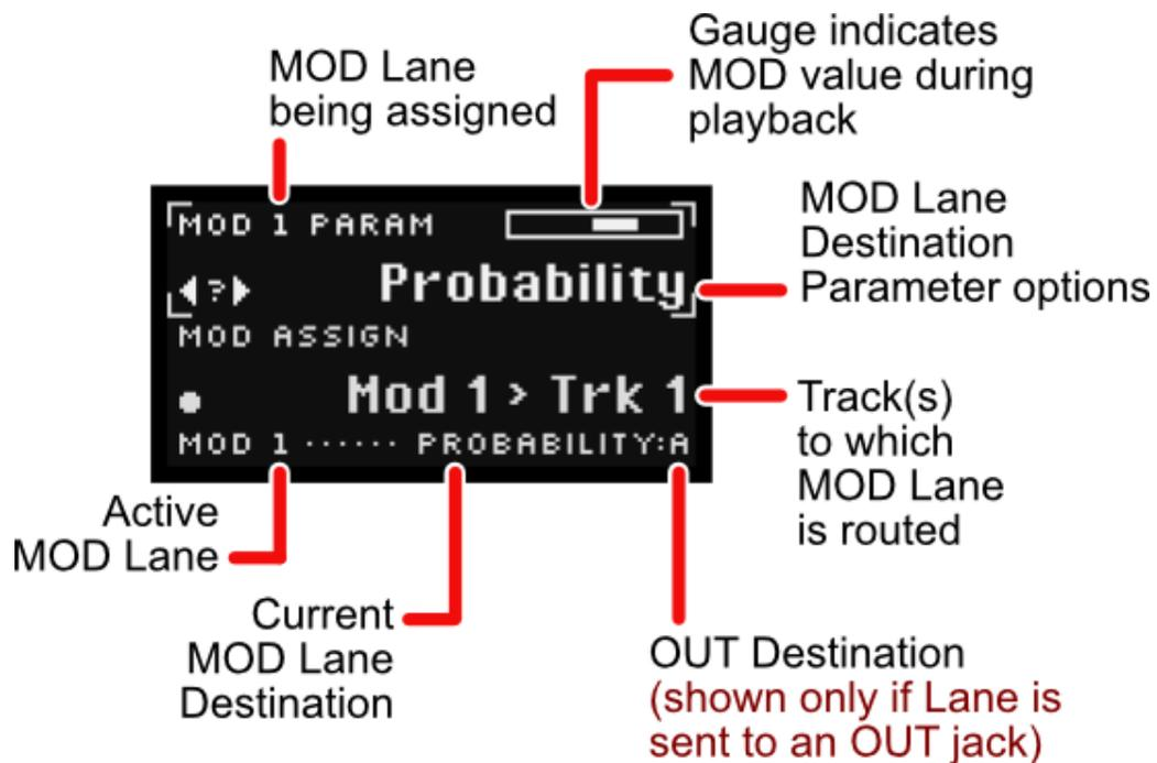
At the top of the screen is a small gauge displaying the current stage's modulation value. Bars extending to the right of center indicate positive modulation, while bars extending to the left of center indicate negative modulation. Any modulation assigned to a trigger or gate function will display a gate icon instead, so you always have visible feedback of your modulation effect.
