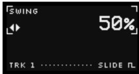
This button opens the SWING screen, which (for the selected track), sets the swing amount between successive clock pulses. Swing delays each even numbered clock pulse by a percentage of the current clock interval. With a value of 50%, no swing is applied (straight time). The more you increase the swing percentage above 50% the more your music will have a 'swing' feel. Metropolis' supports swing percentages from 50% to 78%.
