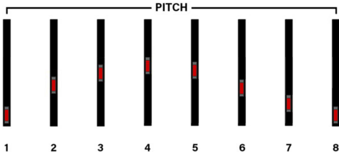
These sliders determine the default pitch value of each corresponding stage. Metropolis uses the position of these sliders as a starting point for determining the actual pitch output by each stage on each track.
