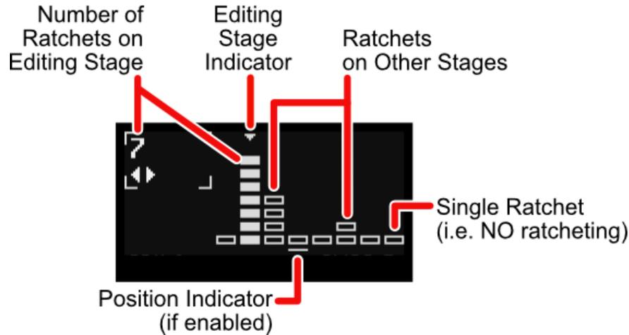
Each stage has a ratchet count from 1 to 8, and the interpretation of this count depends on whether or not **Gate Stretching** (as set in the [Track Menu](#)) is **ON** or **OFF**, as discussed later in this section.
