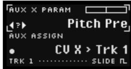
*NOTE: Notice the small rectangular gauge at the top of the AUX Settings screen. This will graphically indicate the amount of post-attenuated CV being applied. Bars extending to the right of center indicate positive CV, while bars extending to the left of center indicate negative CV. Any AUX inputs assigned to a trigger or gate function will display an on/off switch (rather than a continuous voltage bar), so you always have visible feedback of your AUX input's effect.*
