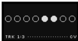
A high gate value (+5V) is indicated by a solid dot (along with a lit **pink** Stage button, when viewing the CV Lane). A low gate value (0V) is indicated by a hollow dot (along with an unlit Stage button, when viewing the CV Lane).
