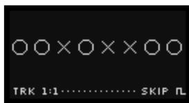
All skipped stages will have an **ORANGE** Stage button. Buttons are not lit for any stages with skip turned off. The screen will also update — showing an "X" for any skipped stage.
