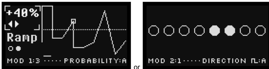
Each MOD lane can have its own playback ORDER, LENGTH and clock DIVision, but the three track timing buttons (SWING, SLIDE and GATE) are not used.
