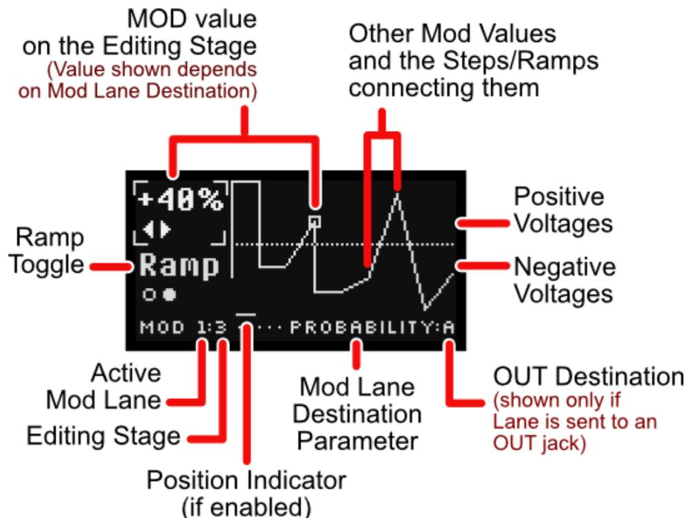
*NOTE: If you have not yet assigned a MOD Lane Destination (discussed in [Assigning a MOD Lane to an Internal Parameter](#)), or if you assigned it to OUT A or B, the editable MOD Value range is +-5.00 V. If the MOD Lane destination controls a variable parameter (rather than a gated parameter), then the MOD Lane Edit Screen works as shown above. If you've assigned a MOD Lane to a gated destination, the MOD Lane Edit Screen works as described in [Editing Gates in a MOD Lane](#).*
