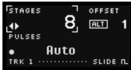
This button opens the LENGTH screen, which controls the sequence length (using a combination of both stage and pulse counts) for the currently selected track.
