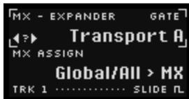
There are two main parameters on the **MX** output assignment screen:
