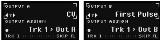
There are two main parameters on each of the OUT (**A** and **B**) assignment screens:
