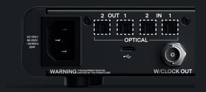
Running in S/PDIF mode, the optical i/o provides the option to integrate external digital outboard, allowing up to 4 channels of audio in and out of the EVO 16 at sample rates up to 96KHz.
