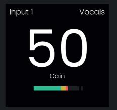
When an input is selected, the hardware will now control that channel, so you can use the Control Wheel to adjust the input gain with decibel level accuracy, as well as toggling channel mute, phantom power for condenser mics, or instrument mode for guitars and basses on channel 1+2.
