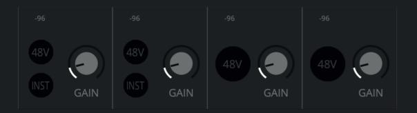
The +48v button will enable phantom power on this channel and the Gain control will adjust the gains on the EVO 16 itself. Allowing you to make quick changes to your setup without having to look away from the computer during a busy session.
