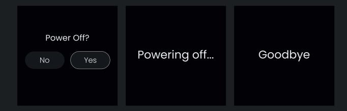
This will put EVO 16 in a low-power standby mode. To turn the unit back on, hold down the Control Wheel until the screen illuminates.
