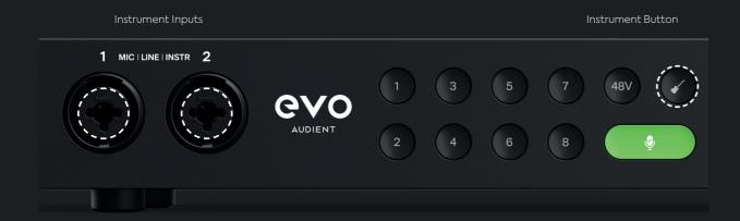
To do this, select either channel 1 or 2, then press the Instrument button. The button will then illuminate as well as display the temporary popup on screen. To turn off Instrument mode, press the Instrument button again.
