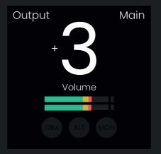
To quickly mute an output, hold down the channel button until the Mute screen is shown, and the channel button begins flashing. When a channel is muted, the volume level is replaced with the Mute icon, this will remain in place until mute is deactivated, by again holding down the output button.
