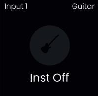
If you try and activate phantom power on Channels 1+2 whilst the instrument input is active, an error screen will show as it is not possible to have both active at once.
