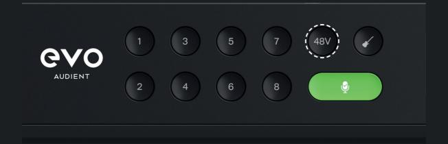
To activate phantom power, select the channel, then press the 48V button, which will then illuminate red as well as activate a temporary popup on screen.
