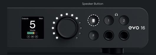
Pressing any of the hardware Output buttons will bring up the Output Status Screen. Similar to the Input Status Screen, with a few key differences, the Output Status Screen displays: the output name, the volume level, stereo meters, as well as a feature status display. With an output selected, the Control Wheel will now control the volume of that output, ranging from 0 to 100.
