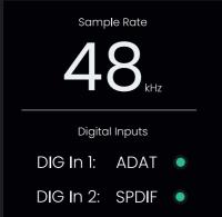
If the light is green, this means that the unit has been successfully clocked, if amber the unit is receiving a signal but in the wrong sample rate, and if red, no signal is detected. To dismiss the screen, press the Control Wheel.
