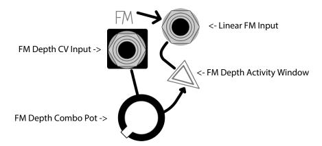
The **Linear FM** input is well suited to audio-rate FM via other VCOs, fast cycling functions from MATHS, or self-patching from the XPO itself. The input is normalled to a version of the Sub Oscillator output, which allows for the superimposition of subharmonics without the need to mix in the Sub-Oscillator with the other waveform outputs.
