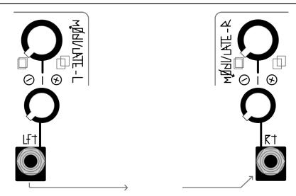
The three stereo output pairs (PWM, Vari-Timbre, Wavefolding) are each affected by the **Modulate L/R** controls in a unique way (see **Stereo Outputs** above for more information).
