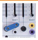
Set all the knobs, switches, and sliders to the default quick start settings from Patch A, but unlike the quick start settings on quick start Patch A, don't connect a shorting bar to the level 2 CV in jack.
