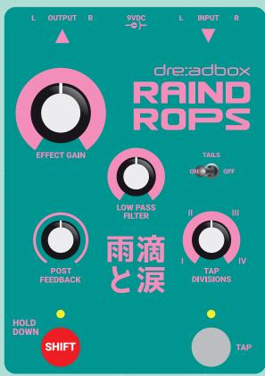
These are the **SHIFT** controls, that you can access while holding down the ON button. Remember, in order to store this so that the pedal remembers them the next time you power it, you must press and hold both footswitches for 3 seconds!
