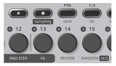
In the example above, the secondary functions of the  ${\stackrel{\hbox{\tiny TD}}{\rightrightarrows}}$  and  ${\stackrel{\hbox{\tiny ID}}{\partial}}$  buttons are "save" and "FX" .
