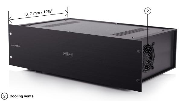
Amplifier draws cool air from each the side of the amplifier case, with hot air exhausted from the top vents of the enclosure. To ensure uninterrupted airflow and the lowest possible operating temperature, it is advisable to leave at least 1U of space on top of the unit. Ultra low noise fans are used to minimize noise. Keep the side vents clear to allow full air flow
