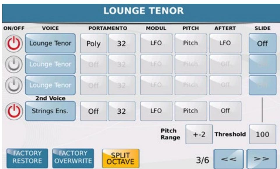
On the third page you may set for each layer the parameters of the **PORTAMENTO** effect (Portamento On/Off and speed), the parameters of **MODULATION** (you may decide to which functions the Pitch Bend and Modulation wheel is applied), and the parameters of the **PITCH** and **AFTERTOUC**H. The **SLIDE** function is also available for the first three layers, where you may set the Threshold value, namely the efficiency threshold of the slide.
