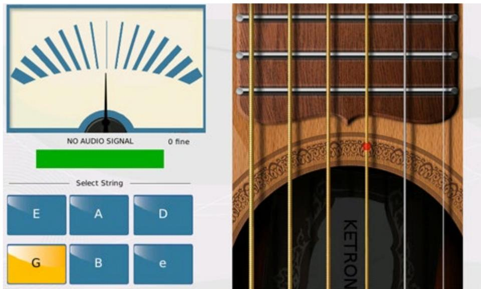
The Tuner mode detection allows to use the tuner instead of the traditional way. By connecting your guitar on dedicated input (MICRO 2) you can check on display current status of tuning. The bar with the GREEN colour will indicate perfect tuning.
