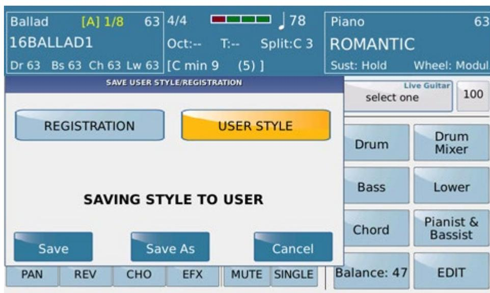
On this page you may save the modifications made to a Registration or User Style. To save the modifications with the current name of the Style or Registration press **SAVE**, or enter a new name with **SAVE AS**: in this case
