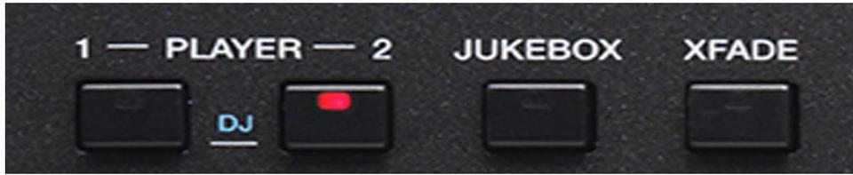
you can enables the **DJ** function that allows an alternative way of playing the songs.
