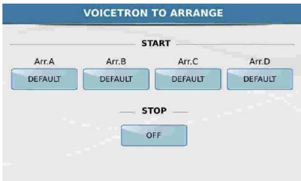
Touch the corresponding box to assign the relevant preset to the 4 Arranges. Off disables harmonisation.
