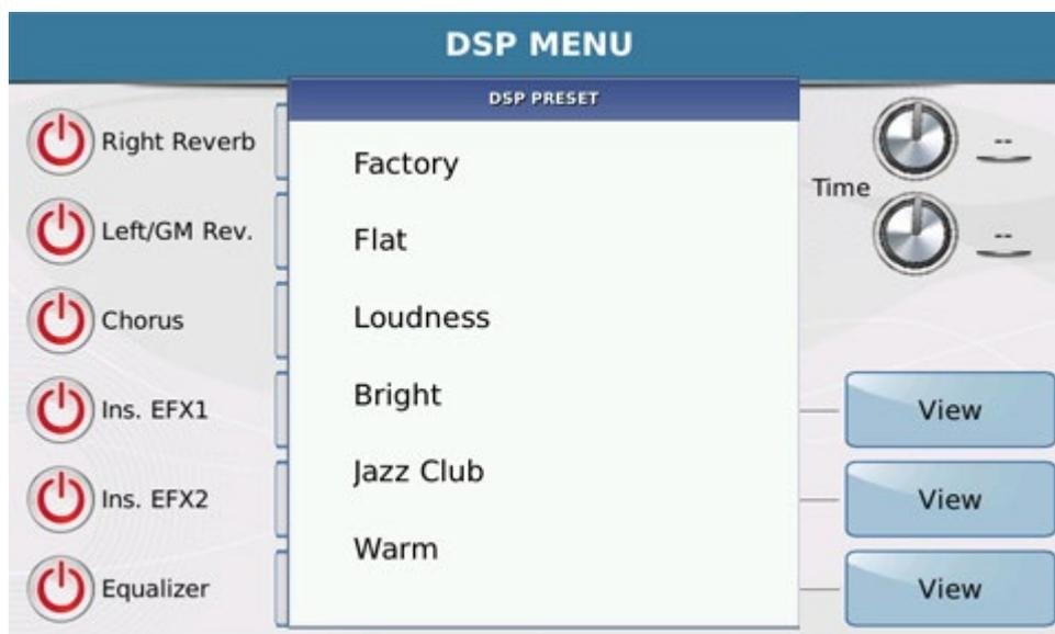
The rectangular box displays the equalisation presets available while the key **View** opens a screen on which you may adjust the equalizer.
