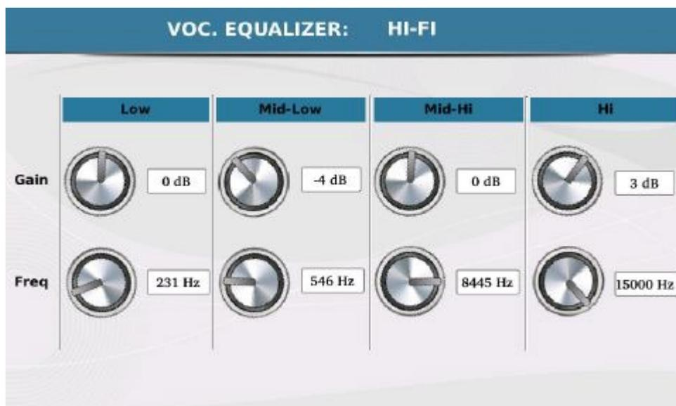
Once you have selected the virtual knobs and modified the value with the Dial, you can save the current preset of the equalizer by pressing the **SAVE** key on the panel and confirming with **YES**.
