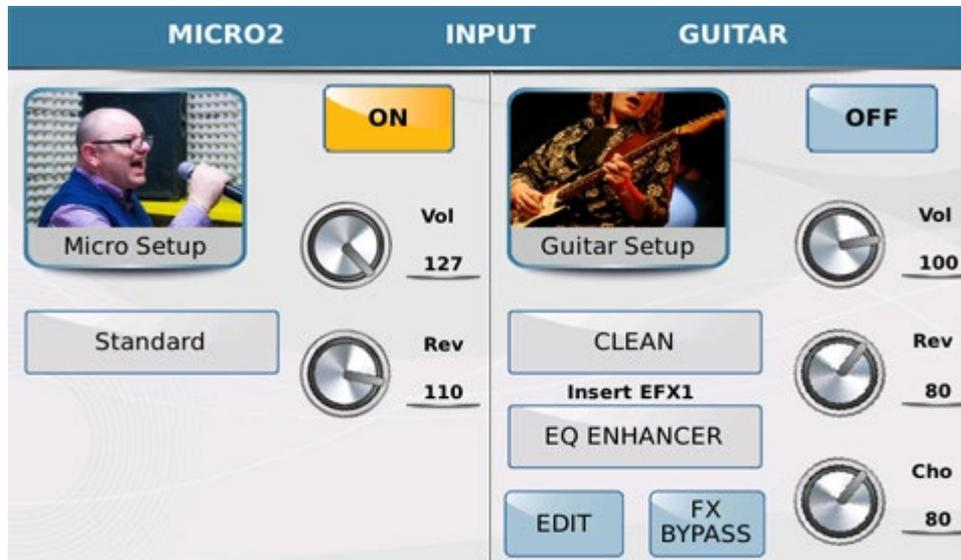
Here again the page is subdivided into 2 sections: the first is **MICRO2** and is for the microphone settings while the second is **GUITAR** and is for the guitar effect settings. Considering that this is a single audio input, the modes cannot be enabled together so that you may either use the input as a second microphone input or as a guitar input. When you enable MICRO2 therefore, GUITAR mode is automatically disabled and vice versa.
