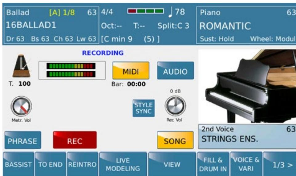
From this menu SD90 can record on Midi mode (and Audio also) everything is played in real time from the keyboard (Left part, Right part or Full Keyboard) .In addition can record ARRANGER section also. The mode displayed on this picture is called SONG Mode. With it user can record freely (dependently of available memory) all notes, change of Voice, Controllers and else.
