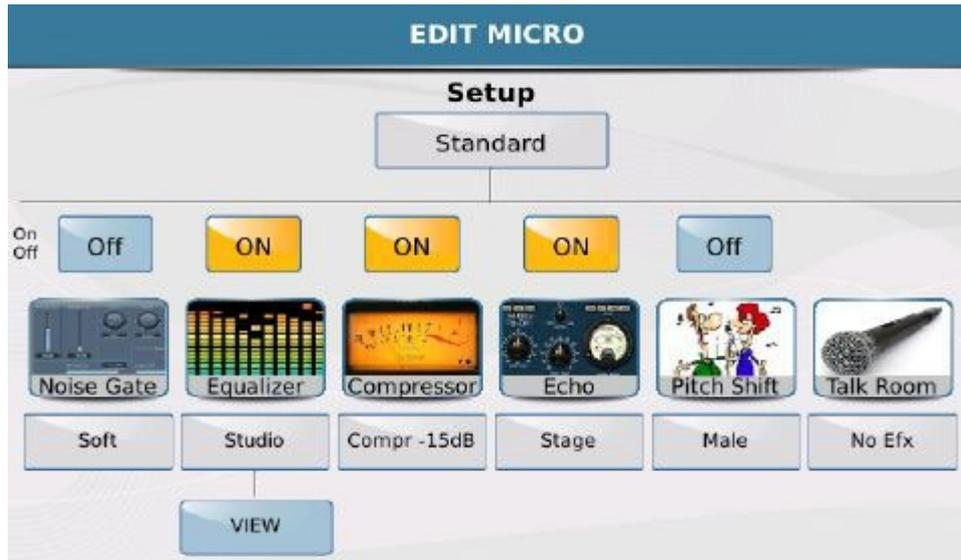
The microphone preset, whose name is displayed in the top box, consists of a number of effects that may be enabled or disabled using the **ON/ OFF** box above the corresponding image.
