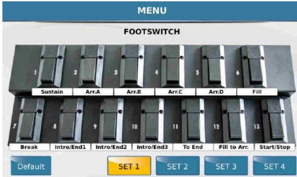
Many functions of the SD90 may be assigned to optional footswitch controls FS6 (6 switches) or FS13 (13 switches).
