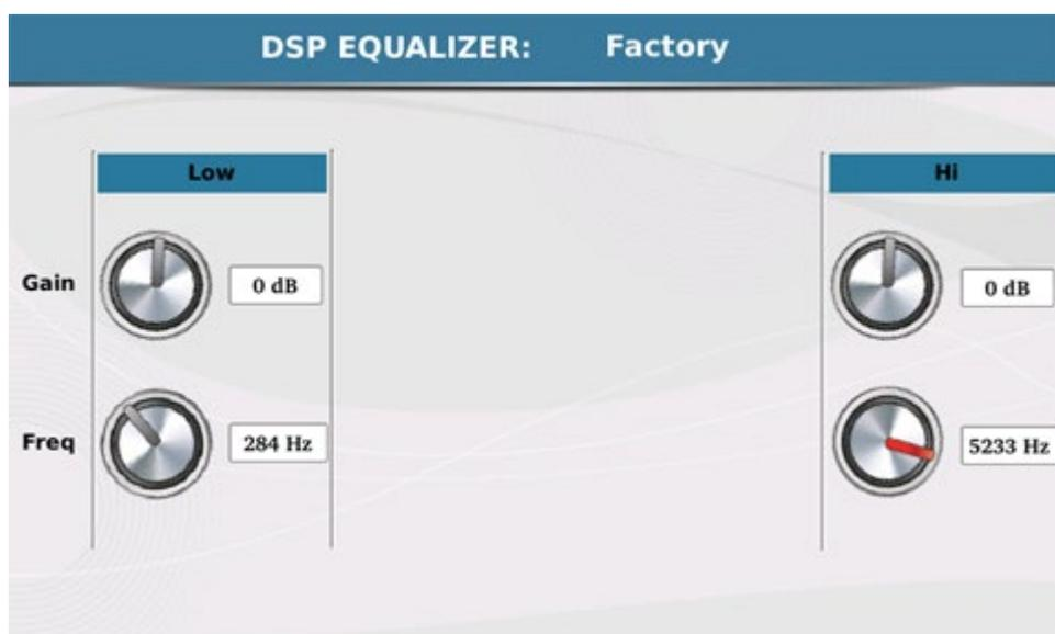
On the left you will find a box on which you may adjust the Lows, where the upper knob is used to set the level and the lower knob is used to set the frequency at which the level is applied. The steps to follow to make this adjustment are the same: select the knob on the display and turn the Dial left or right.
