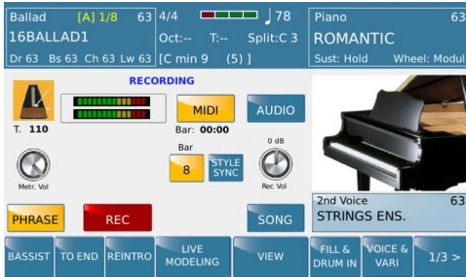
If set, as showed on picture, a number of 8 measures by using Bar tab on PHRASE mode SD90 will record just only up to 8 measures. This action will force to exit automatically from the method RECORD when 8 measure bar will be terminated
