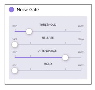
Lion's noise gate silences extraneous noise generated by these high gain tube amps by detecting your guitar signal at the input, but acting at the end of the signal chain. This clever design is extremely effective at both detecting and stopping extraneous noise.
