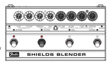
To set the pedal to Original Blender Mode, turn on the effect (indicated by the Bypass Footswitch LED illuminating red) and press the Octave Footswitch until the Octave Footswitch LED illuminates red. The Octave Footswitch LED will remain illuminated red even when the effect is bypassed to indicate the mode of the pedal when you turn it back on. Pressing the Octave Footswitch again will change the pedal to Octave Blender Mode.
