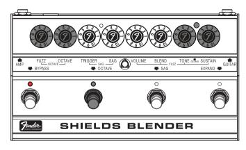
To set the pedal to Octave Blender Mode, turn on the effect (indicated by the Bypass Footswitch LED illuminating red) and press the Octave Footswitch until the Octave Footswitch LED illuminates white. The Octave Footswitch LED will remain illuminated white even when the effect is bypassed to indicate the mode of the pedal when you turn it back on. Pressing the Octave Footswitch again will change the pedal to Original Blender Mode.
