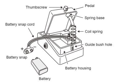
Hold down the pedal and loosen the thumbscrew, then open the pedal upward.
