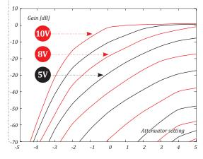
fig. 5: GAIN RESPONSE TO CV
