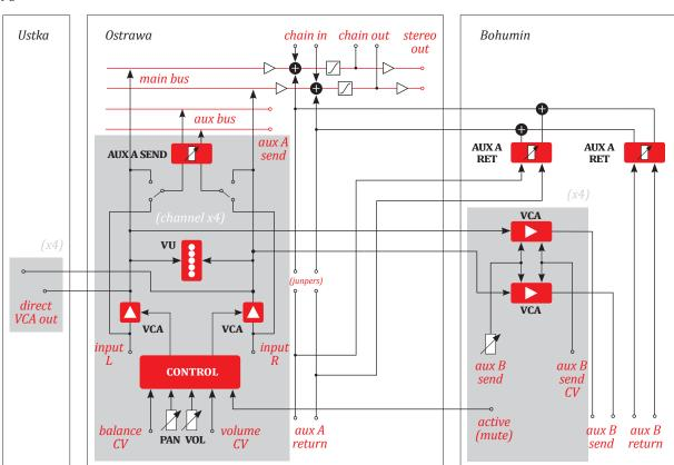
fig. 1: OSTRAWA, BOHUMIN & USTKA SIGNAL FLOW
