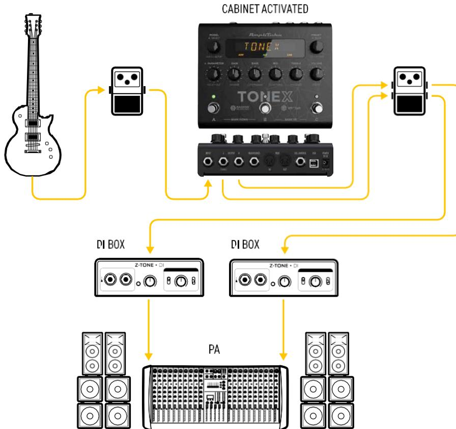
This is an example of using the pedal alone with a PA System in stereo:
