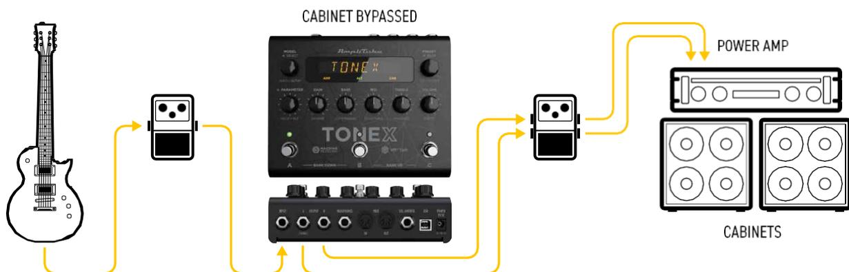
This is an example of using the pedal alone connected to a power amplifier feeding a guitar or bass cabinet:
