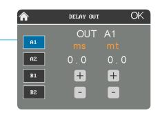
The Delay page allows users to independently set the delays for the four output channels (up to 3.5 mt) and for Channel 3 and Channel 4 input channels (up to 114 mt).
