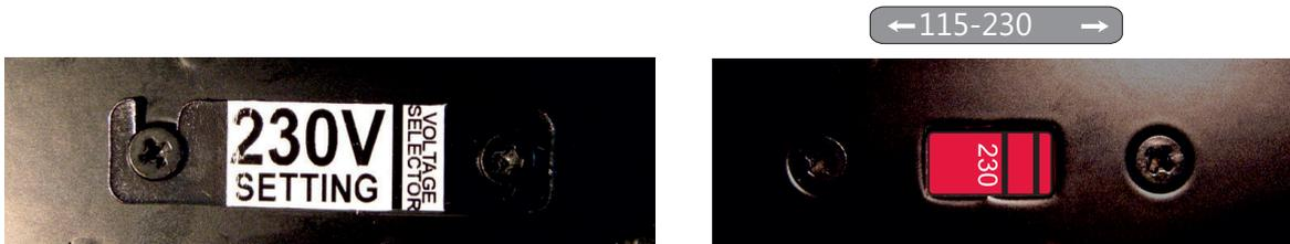
The device is default set to be connected to 230 V AC Power. To use the device on a 115 V AC Power you need, before connecting it, to move the voltage selector's cover, just loosening the two screws, and to choose the correct use voltage by the red switch. Be sure that both voltage set on the selector and AC Power have the same value. Always close the voltage selector's cover before connecting the device to AC Power. Change the label that points out the correct voltage in use.
