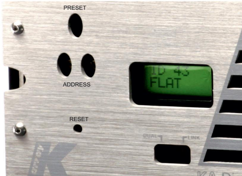
order to remote your system, you need to set each module on a different address, so that, in your chain, no one module will have the same address. Two rotary encoders allow you to set the desired address number that will appear on the top line of the display. Using the remote control software it is possible to mute each system, select a desired preset loaded on-board or download a new preset pack.
