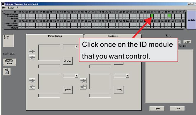
Temperature rectangle red: one module inside that loudspeaker is over-temperature.
